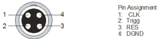
Figure 8 - DEWESoft® 4pin Sync connector
